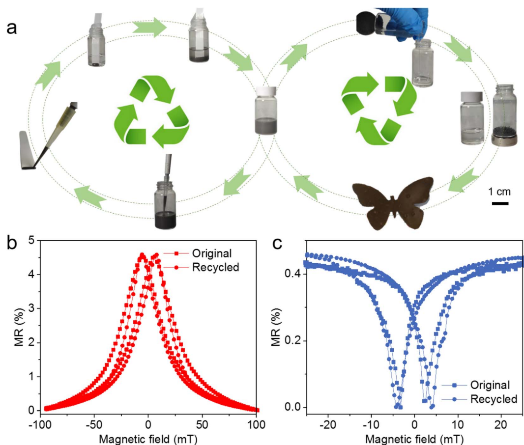
Fig. 4 Recyclable properties of printed magnetoresistive sensors. (a) The left loop illustrates the recycling and reproduction process of printed magnetoresistive sensors: discarded sensors are immersed in solvent to decompose magnetoresistive fillers and polymer binders, after which the recycled ink is used to fabricate new sensors. The right loop illustrates the separation of component materials and the fabrication of a magnetic soft robot using the separated polymers and magnetic fillers. (b and c) MR response of the printed sensors with the recycled materials. The sensors exploit (b) GMR microflakes and (c) AMR microparticles as fillers.
